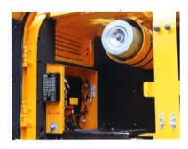
Centralized Electric Control Box and Easy Change Air Cleaner Assembly
